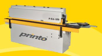
Panel movement system by means of top powered feeder, reliable toothed belt Machine base made of steel: stable and rigid, keeping the adjustments Front telescopic support with roller conveyor for bigger work piece Glue temperature electronic control with digital read-out Friction free work table with six rollers. Easy adjustment of trimming and buffing units.
